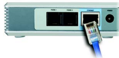
Figure 3-3: Connect the Ethernet Network Cable
