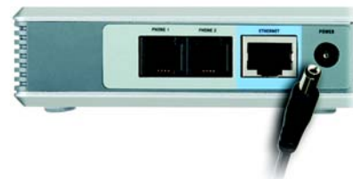
Figure 3-4: Connect the Power
